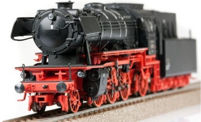
When buying a new or second hand model train locomotive always carefully check the wheels. When not connected to a gear, the locomotive wheels will move easily when prodded with a finger. The wheels on a locomotive may move just a little and then go stiff. If that happens it is usually an indication the wheels are connected to a gear. That's a good sign.
