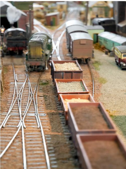
A flickering locomotive headlight can point to a dirty track. Be careful cleaning track with harsh abrasives because if you remove the smooth coating on the track it will be exposed to oxidation and will need cleaning more frequently. The track collect dirt and grime more easily.
